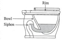
The toilet works by a simple mechanism based on gravity. The bowl is attached to a pipe with an S-bend to the sewer. Activating the flush lever lifts a
